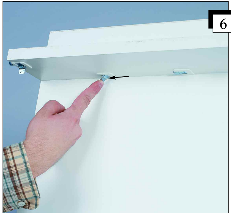
6 Once the toe and bottom panels are together, press the fitting toggles down to secure.
