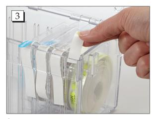
**Step 3.** Pull out the first few labels on the roll and slide them down into the label guide on the front of the dispenser. (The first couple labels will need peeled by hand.)
