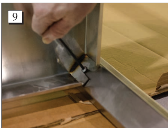
Step 9. Tighten the button head screws on each leg with the provided Allen wrench.
