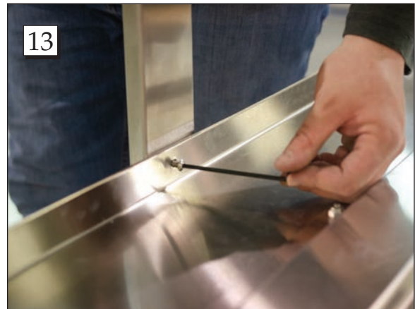
Step 13. Then secure the middle legs to the shelf with one button head screw on the inside of the leg.
