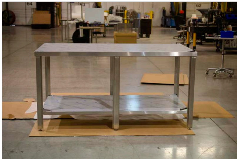
Step 12. Secure the middle legs to the top with a button head screw on the inside and outside of each leg.
