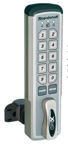
To operate the Self Lock version of RegulatoR: Type a valid code, press ENTER and rotate knob clockwise 90°, hold knob until door or drawer is open. Release knob, RegulatoR knob will return to the locked position. Door or drawer can be closed at any time.
