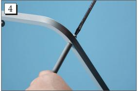
**Step 4.** Use a flat head screw driver to tighten the rail in place.
