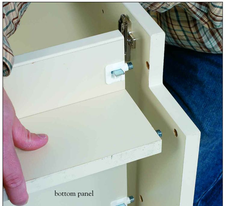
7 Attach the right side by aligning the pre-drilled holes with the connection fittings in the back, bottom and top panels.
