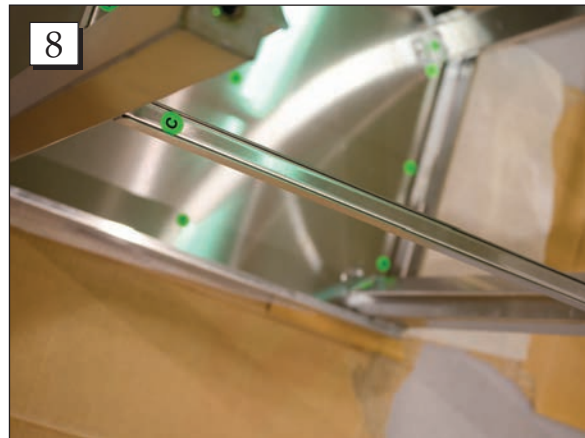
Step 8. Place the long support bars marked "C".
