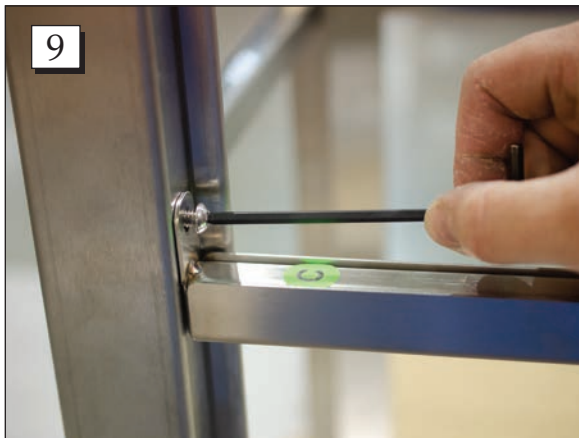
Step 9. Secure each side of the long support bar with a button head screw. Tighten the button head screws with the provided Allen wrench.
