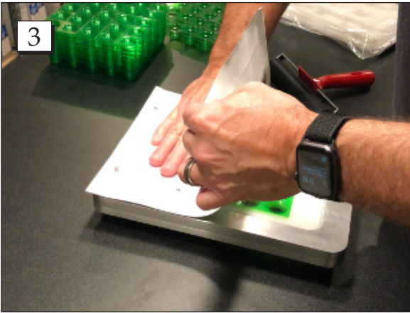
Step 3. Place the labels onto the locating pins and gently lay the labels onto the blisters.
