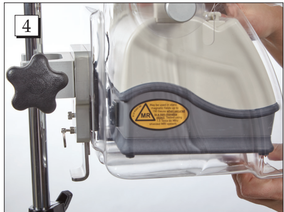
Step 4. Roll the pump into place. Note: When properly seated the pump cannot be lifted out of the locking mount.
