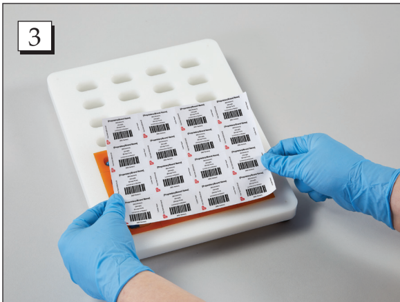
Step 3. Peel the prepared labels from the 8½" x 11" sheet. Hold them by the edges and apply the label strip to the blisters in the sealing tray.
