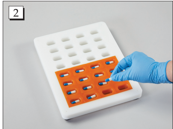
Step 2. Fill each blister cavity with a tablet or capsule.
