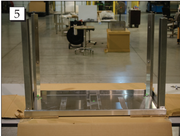
Step 5. Repeat steps 2-4 on the remaining legs marked "D".
