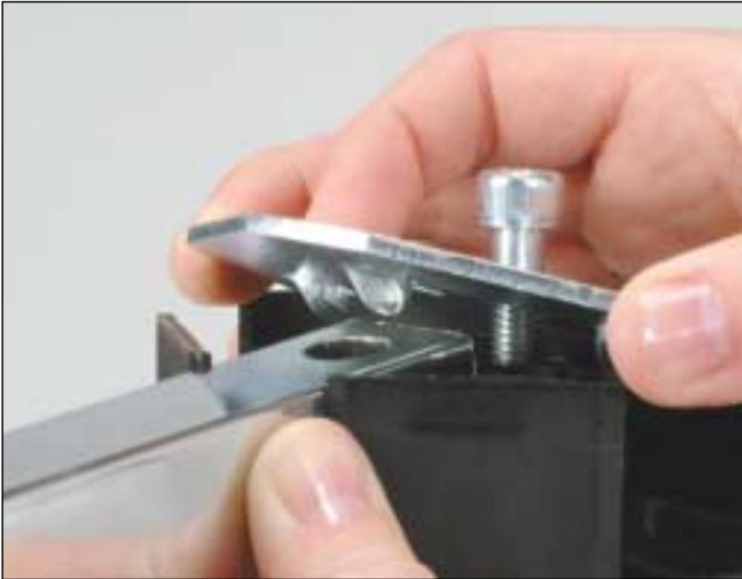
9. The grooves of the clamp disk must fit in the holes of the feet so that each foot is locked into the 5-footed plastic mid-section before tightening.
