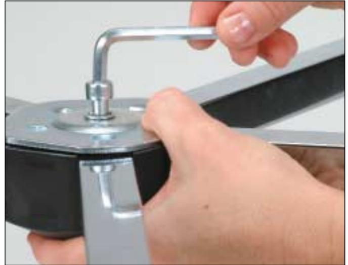
10. After all five feet have been placed into the plastic five footed mid-section, tighten the cheese-head screw by turning it clockwise with the wrench provided.
