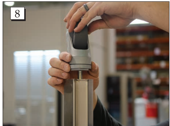
Step 8. Tighten the four casters into place.
