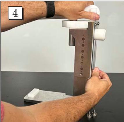
**Step 4.** Adjust the height of the top until the proper position number lines up with the threaded hole. Tighten the thumb screw once at the desired height.
