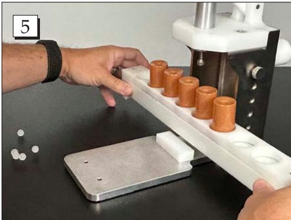
**Step 5.** Fill the vial with the desired medication. Then place the carrier in between the white guide block and the frame. It should move freely to the left and right.
