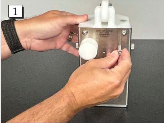
**Step 1.** Remove the 1/4" Socket Head Cap Screw from the back of the unit.
