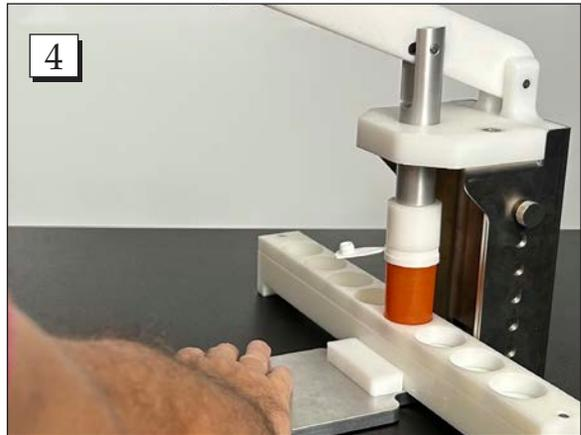
**Step 4.** Press the cap onto the vial with firm pressure.
