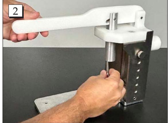
**Step 2.** Thread the 1/4" Socket Head Cap Screw into the bottom of the anvil as far as it will go.
