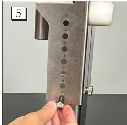
**Step 5.** Reinstall the left and right thumb screws into the position hole (see guide below). Repeat this step for the other side.
