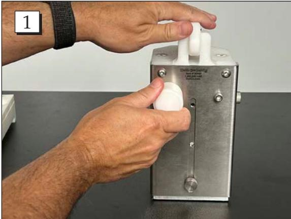
**Step 1.** Remove white the Anvil Insert from the back of the unit.
