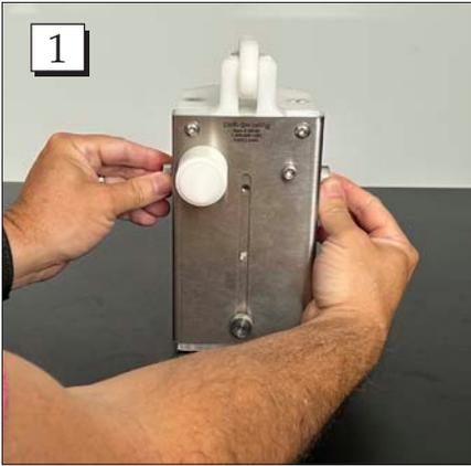
**Step 1.** Remove the thumb screws from the right and left side of the unit.
