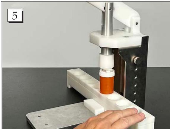
**Step 5.** Fill the vial with the desired medication through the port hole on the top of the cap. Flip the port seal flap over the port opening and firmly press the closure shut.
