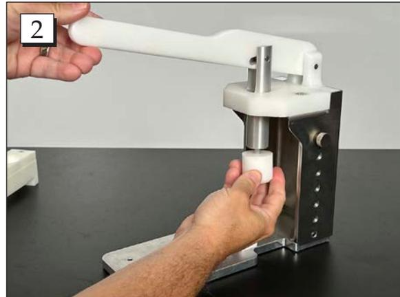
**Step 2.** Thread the white Anvil Insert into the bottom of the Anvil.
