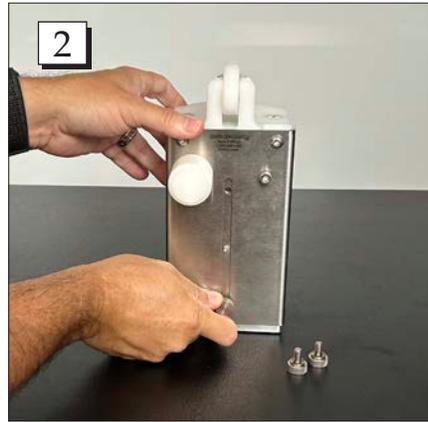
**Step 2.** While holding the top, loosen the back thumb screw until the top can be slid upward.
