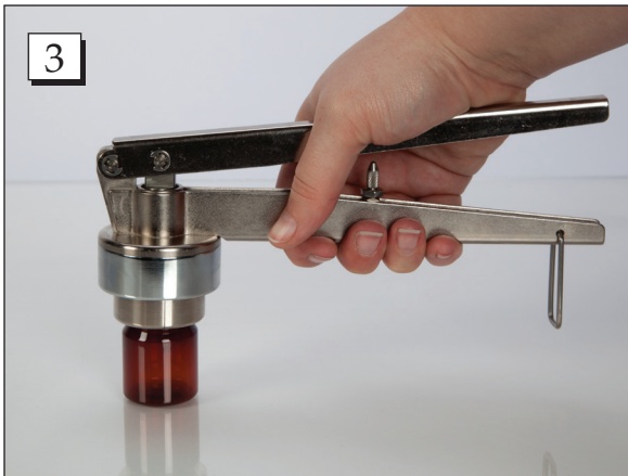
Step 3. Gently squeeze the handle of the crimper to attach the cap onto the vial.
