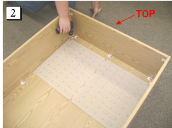
**Step 2.** Line the 1st panel up with the pre-drilled holes starting at the top, and use a screw and washer configuration to secure. (NOTE - make sure louvered panels are upright.)
