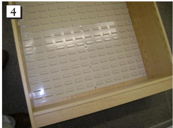
**Step 4.** Repeat steps 2 and 3 until all of the panels are secured into position.
