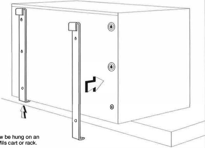
**4** Repeat procedure for second strap. Cabinet may now be hung on an Akro-Mils industrial louvered panel, or on any Akro-Mils cart or rack.
