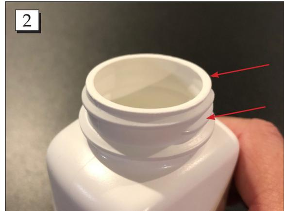
**Step 2.** Make sure the threads and top sealing surface are clean and free of grooves that could create a leak path.
