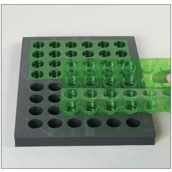
2. Remove two 4 x 6 grids of blisters from the blister stack and place in the sealing tray.
