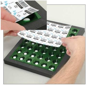
5. Holding the label grid by the edges on either side, apply the to a grid of blisters in the sealing tray by matching the adhesive on the labels with the edges of the blisters. Repeat steps 4-5 for the second grid in the tray.
