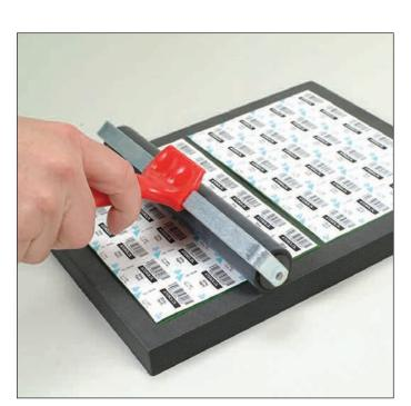
7. Enhance the seal by applying moderate pressure to the sealed blister grids using a sealing roller. Smooth the labels along the entire length of the blister tray.
