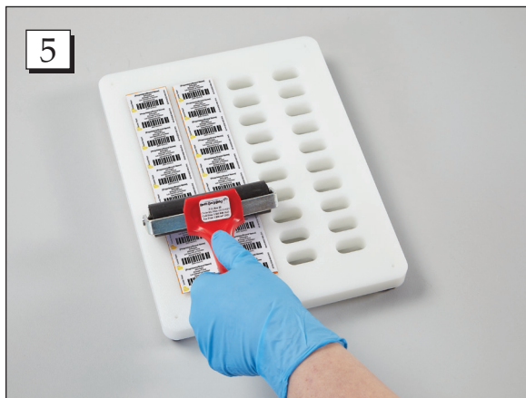
Step 5. Apply moderate pressure with a sealing roller to ensure a secure seal on the blisters.
