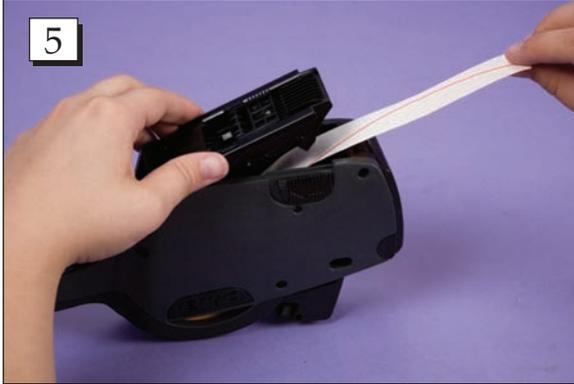
**Step 5.** Pull the tail out and close the bottom assembly.
