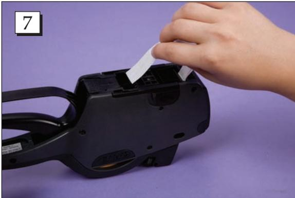
**Step 7.** Feed the tape through the feed drive wheel on the side closest to the handle.
