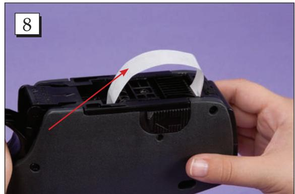
**Step 8.** Be sure to remove the labels on the outside of the gun. Otherwise they will get clogged up when the tape advances through the gun.
