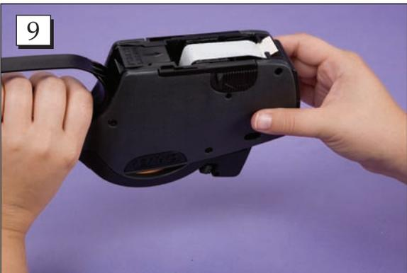
**Step 9.** Click the handle of the gun several times to progress the tape through the gun.
