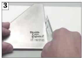
3. Score the strip 3 to 4 times along the straight edge of your template using your retractable knife.
