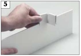
5. Slide your clips onto the edge of your strips by pushing the open end of the clip onto the strip.
