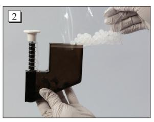
**Step 2.** Plug the hole using the Easy Fill Vial Plug Dispenser, HCL #7339. Fill the dispenser with a bag of plugs.
