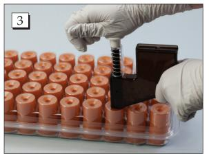
**Step 3.** Position the dispenser over the vial and push down on the plunger.
