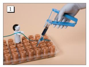
**Step 1.** Using the holder tray, fill the vial through the hole in the bottom using a Dispensing Syringe, HCL #3221 or automatic filling pump. We recommend starting at one end of the row of vials and working systematically down the line, row by row.
