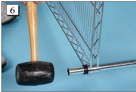
Step 6. Tap into place with a rubber mallet.
