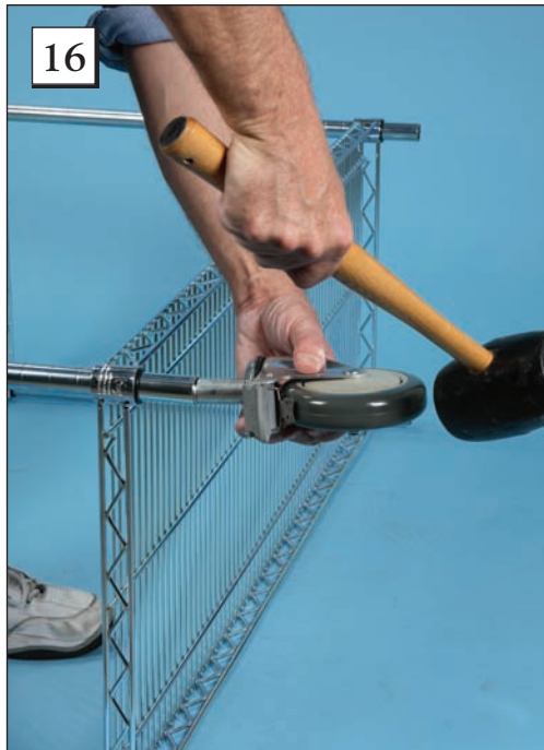
Step 16. Tap a caster into the bottom of the cart with a rubber mallet.
