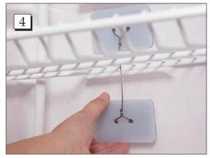
**Step 4.** Align the bottom Acrylic Pad on the back wall of the refrigerator and press firmly to attach.
