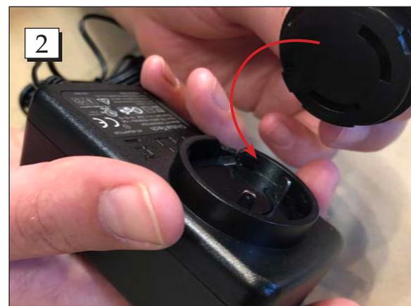
**Step 2.** The AC power supply comes with 3 adapters. Type A, Type C and Type G. Choose the appropriate adapter, place and twist the adapter into place on the power supply.
