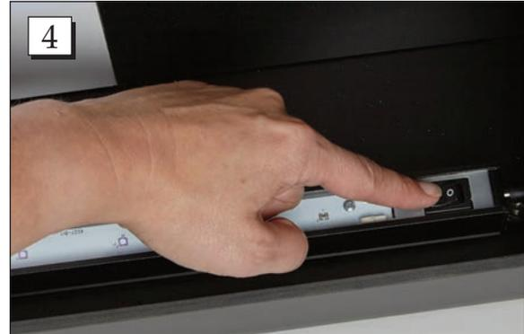
**Step 4.** Flip the switch on each light housing to turn on/off.
