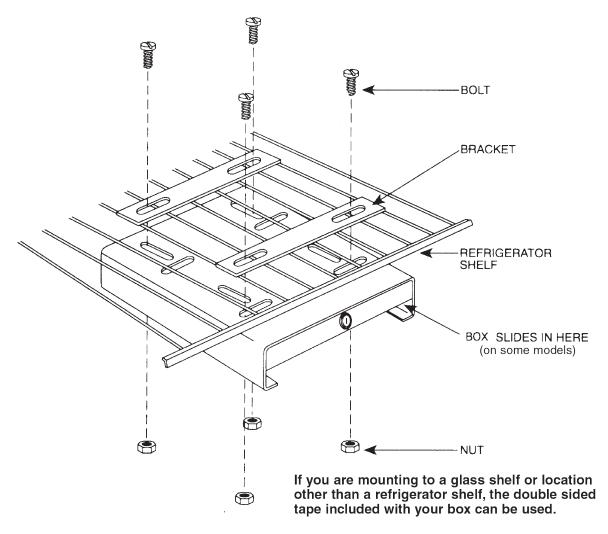
This tray was designed to be attached to wire grid type refrigerator shelves. If possible remove the refrigerator shelf unit on which the box is to be installed. Tools required: a 7/16" wrench or a socket and a wide blade screwdriver.
