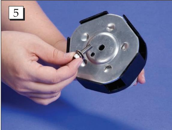
**Step 5.** Insert the screw through the hole on the cover plate into the pole adapter and thread the screw in three turns.
