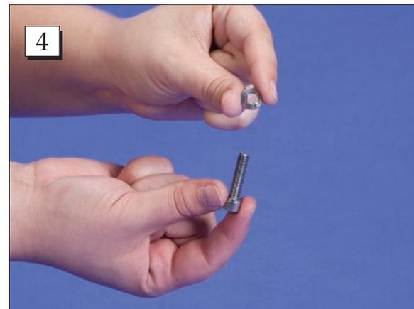
**Step 4.** Place a lock washer first followed by a flat washer over the screw.
