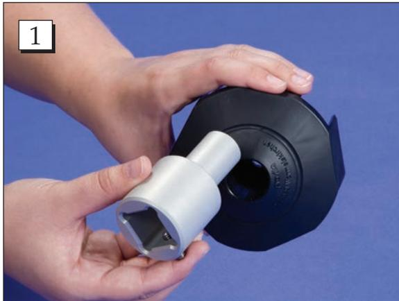
**Step 1.** Place the pole adapter into the black plastic housing.
