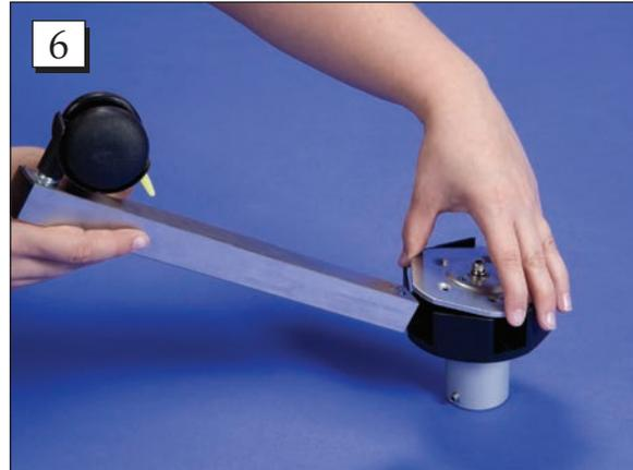
**Step 6.** Tilt the cover plate up and insert a leg section with the open hole in the leg facing upward toward the cover plate.
