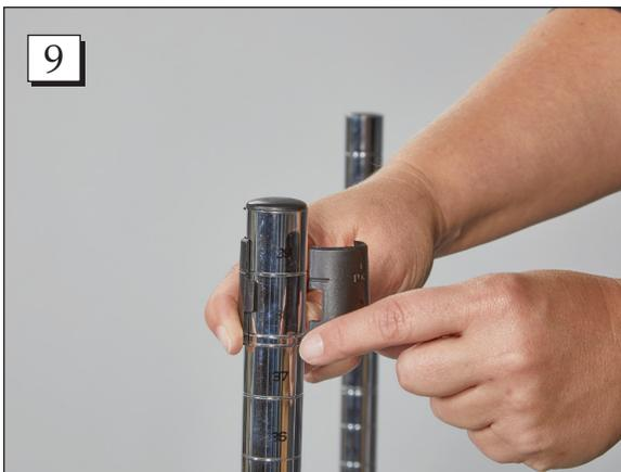
**Step 9.** At the first (top) notch on each post, attach a clip.
