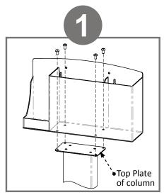
Attach selected accessory to the column using (4x) screws included with stand. Tighten.
