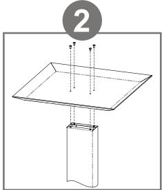
Use Phillips screwdriver to secure base to column with (4x) screws  $(10-32 \times 5/16")$ .
