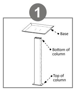
To secure base to column, turn column upside down (with top plate down) and place base inverted, as shown, on column.
